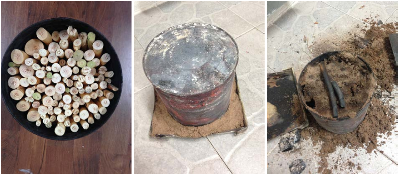
Image 3. Production process of artists' charcoal: charring stages of willow branches, 5 November 2021. Image: Murat M. Türkmen, license CC BY 4.0.
